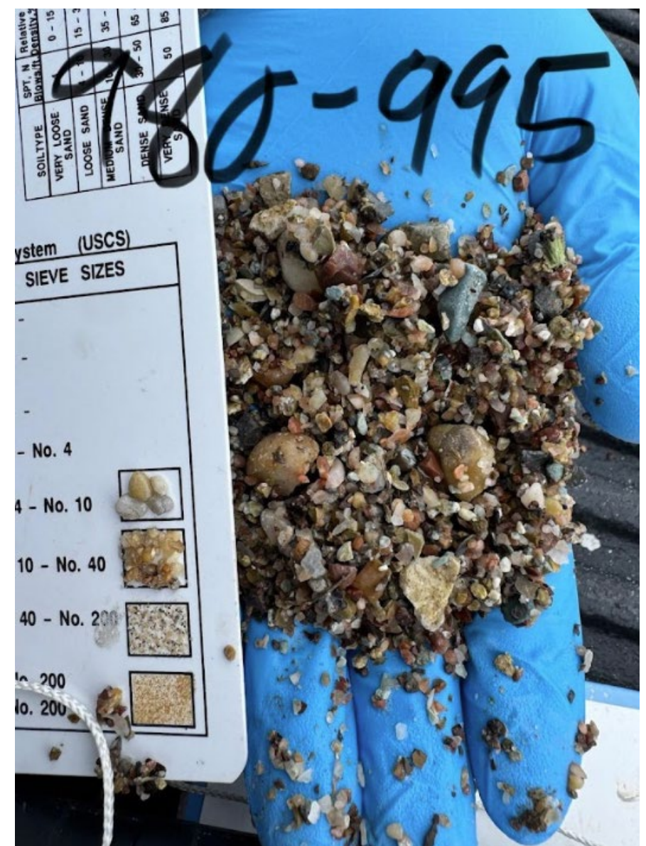
Lithologic Log from Monitor Well Bottom 100'
